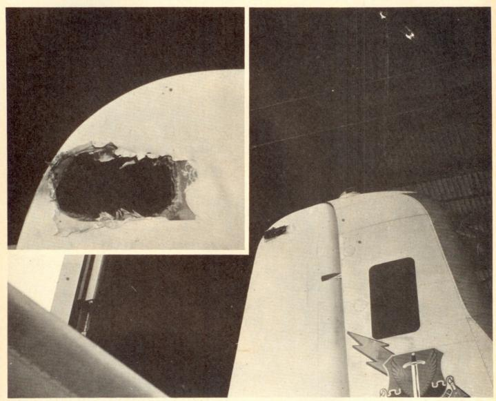
A lightning strike left this hole in the rudder of an Air Force C-118. Photos courtesy of FAA.
